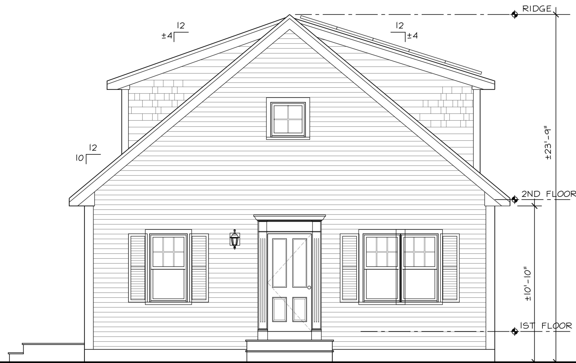
FRONT (STREET) ELEVATION SCALE: 1/4" = 1'-0"
