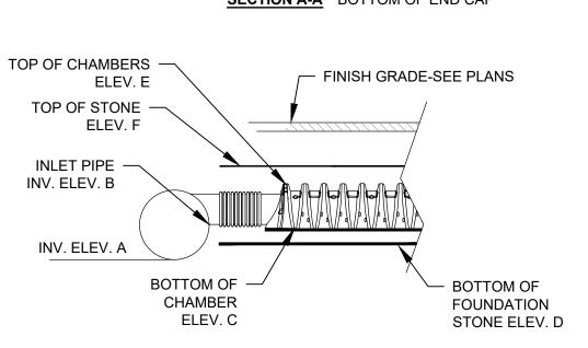
STORMTECH SYSTEM DETAIL NOT TO SCALE
