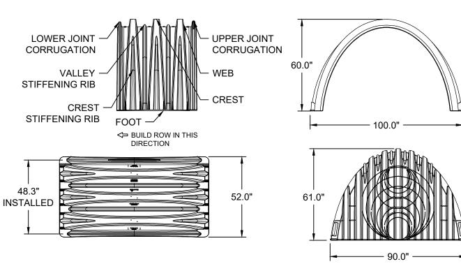
NOMINAL CHAMBER SPECIFICATIONS SIZE (W X H X INSTALLED LENGTH) **CHAMBER STORAGE**
