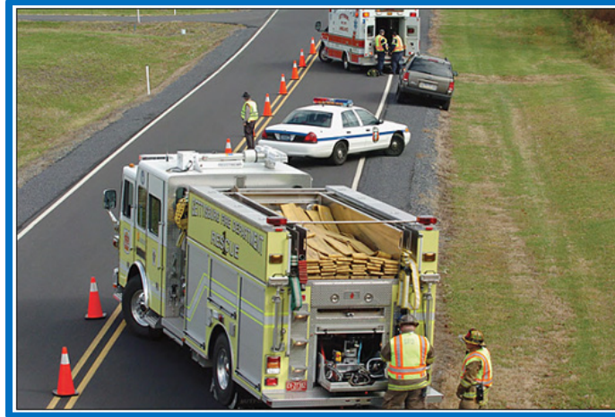
FIGURE IV-20: FIRE APPARATUS SERVING AS A BLOCKING VEHICLE ON A ROADWAY INCIDENT
