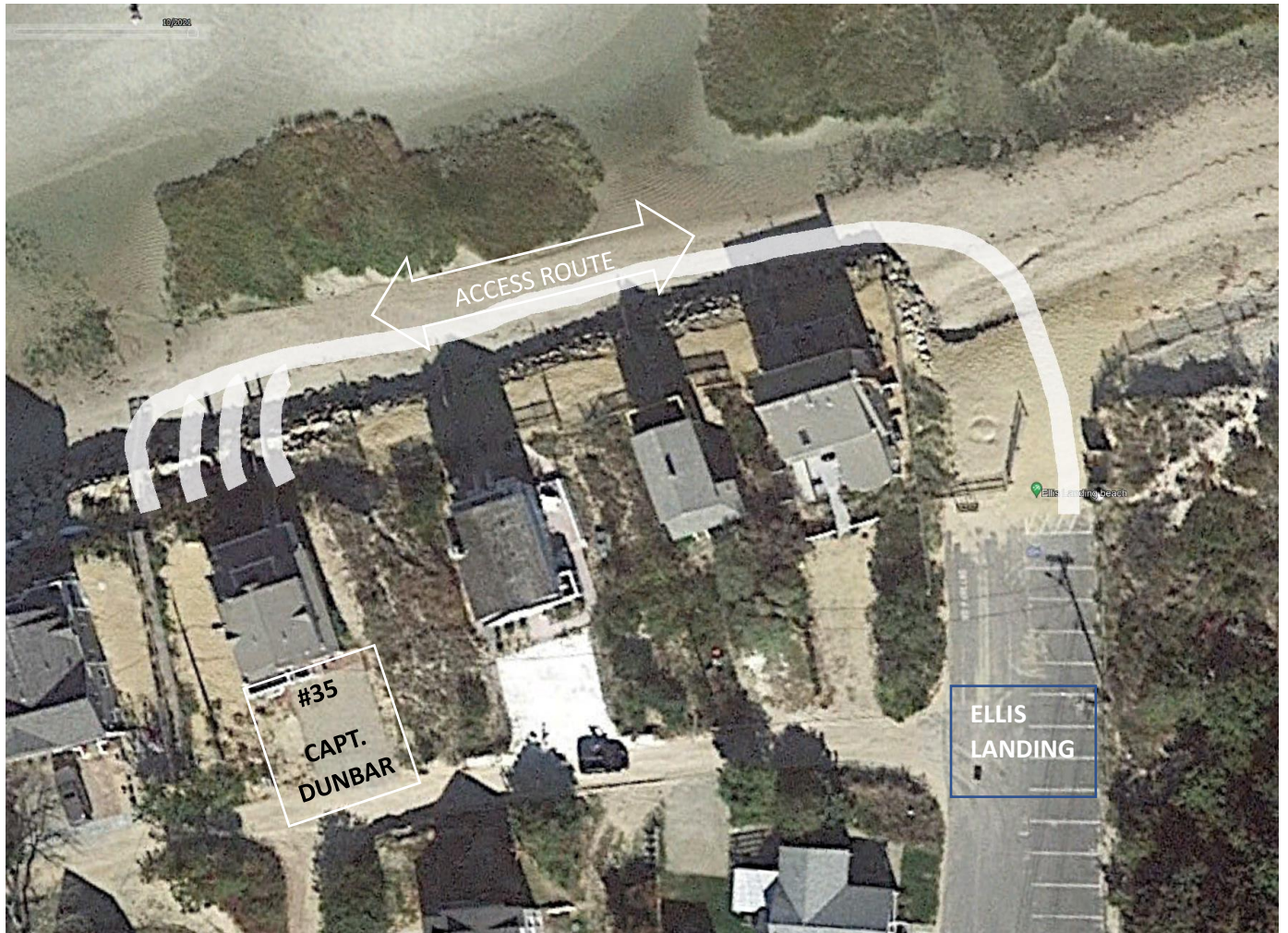
Site Access Map - Sand supply route from Ellis Landing to 35 Capt. Dunbar Road. Staging within Ellis Landing parking lot will be per agreement with Anchor Marine, Inc. and the Town of Brewster.
