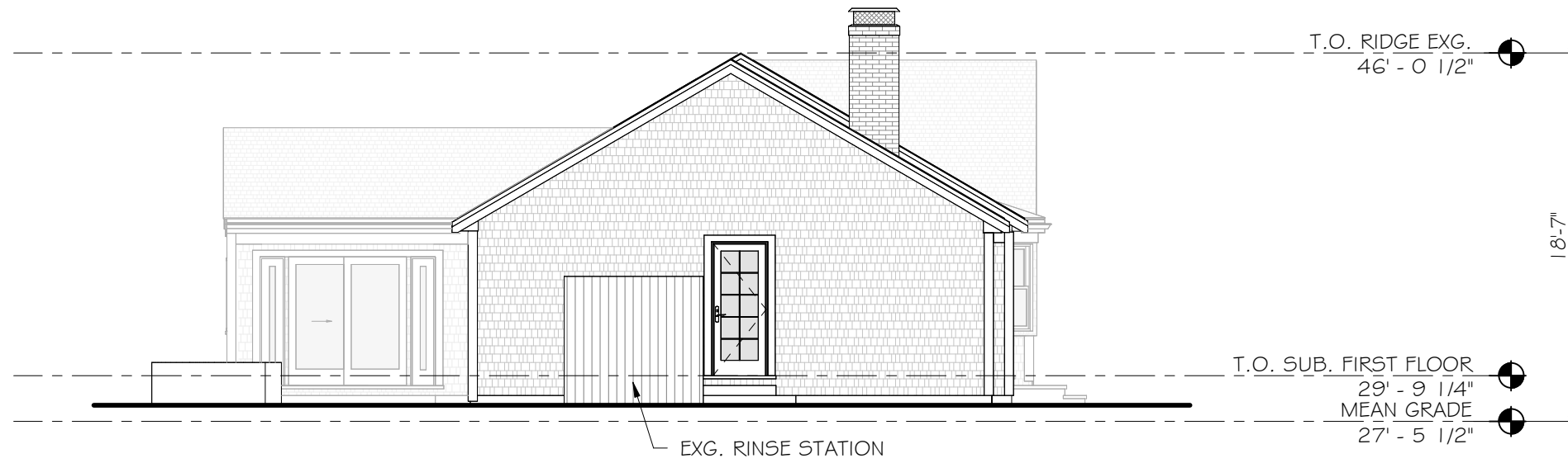
1 EXISTING SOUTH ELEVATION 1/8" = 1'-0"
