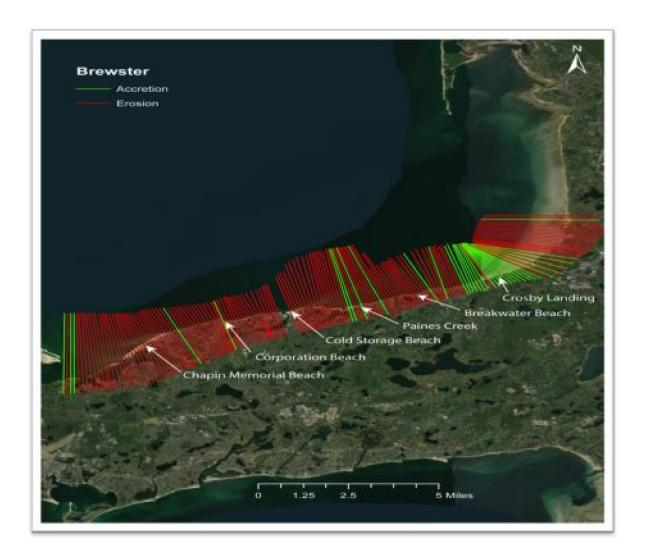
Figure 1 above shows the pattern of erosion and deposition of sediment within the Dennis-Brewster-Orleans littoral cell. The net direction of sediment movement in the littoral cell is from Dennis (a sediment source) to Brewster (a sediment sink). Source: Borrelli
